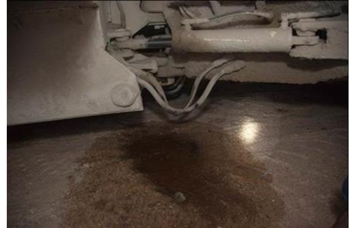
Hydraulic Leak under Sister Vehicle
